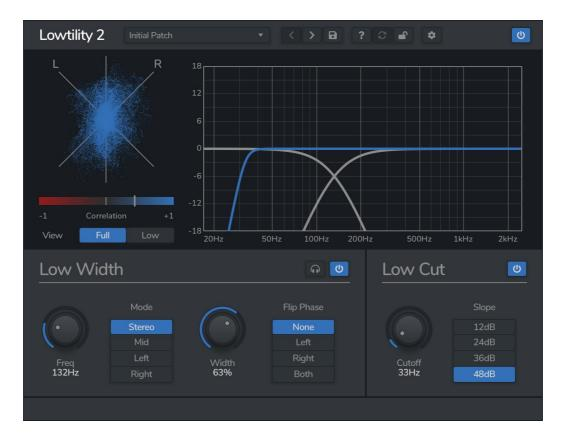
Lowtility 2 is a low-end filter and mid/side utility plugin. Lowtility 2 lets you cleanly cut the low frequencies from your mix, and modify the stereo field. You can cut the low frequencies using a variable slope low-cut filter, reduce the stereo width of the low end, or completely make it mono, using either the mid channels or one of the side channels.
